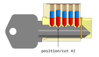
Each chamber holds a **pin stack** — a **spring**, a **driver** and a **key pin**. When a key is inserted, the *cuts* on the key will determine how far each *pin stack* is compressed against its spring. A *working key* compresses all stacks such that all key pins and drivers *divide* neatly along the **shear-line**, allowing the plug to *rotate* freely inside the housing.
