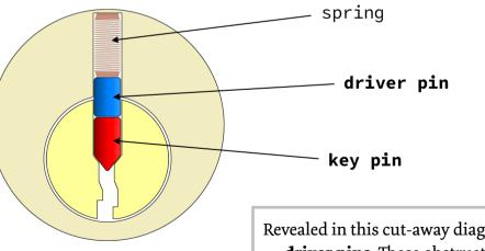
Revealed in this cut-away diagram are further pins — **driver pins**. These obstruct the free rotation of the **plug** inside the **housing** or **shell**.
