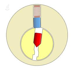
What now? Find the **binding stack** or 'binder' and gently compress the stack without applying too much torque (to avoid seizing up the lock completely). You may have to let off a little tension — just enough — to **clear** or **set** that pin stack. Be careful though: if you let off too much previously-set pins will fall back/reset themselves due to the pin stack's spring!
